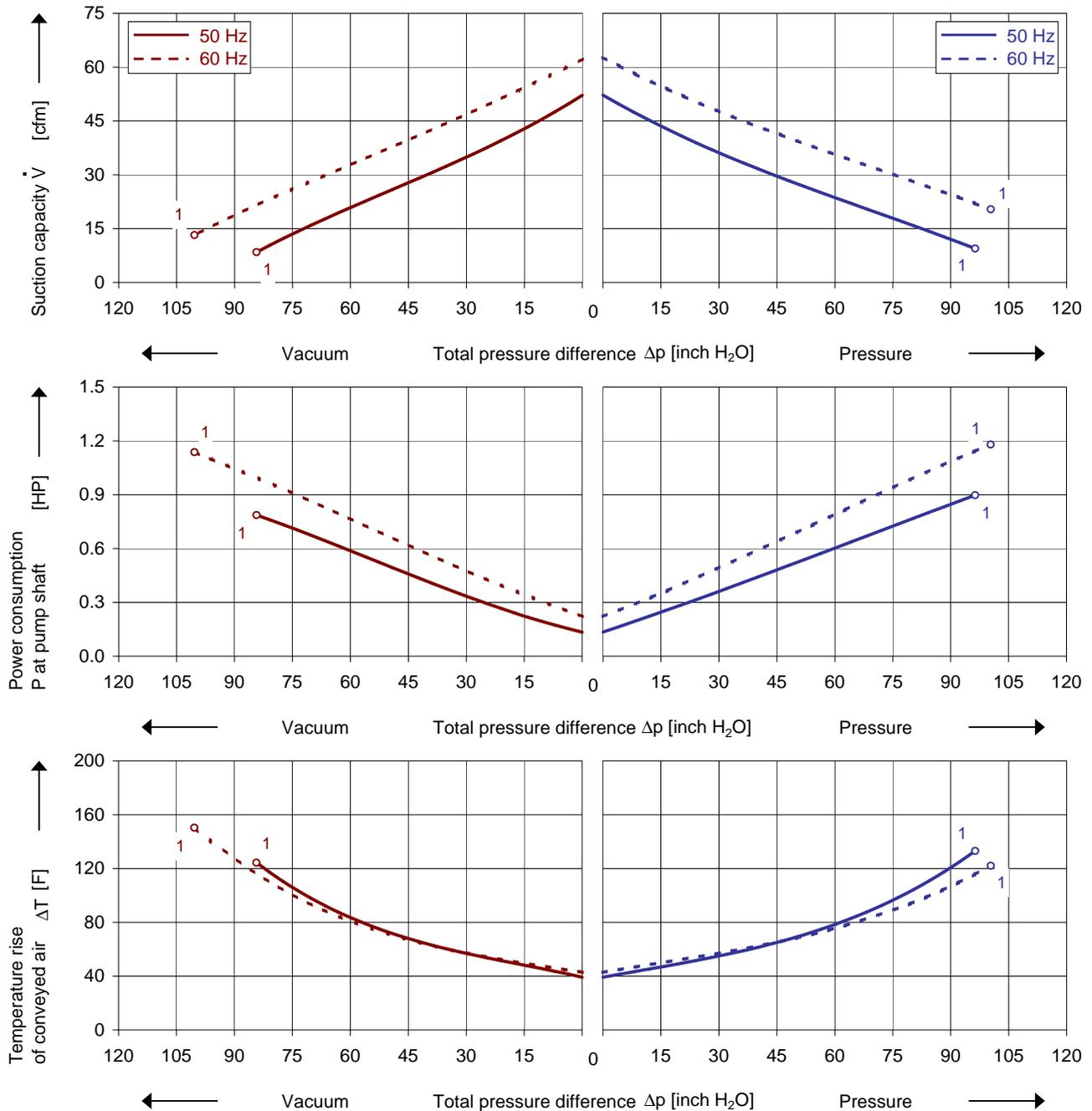
The performance curves are based on air at a temperature of 59 F and an atmospheric pressure of 29.91 inch Hg with a tolerance of ± 10 %. The total pressure differences are valid for inlet and ambient temperature up to 77 F. Suction capacity relates to inlet conditions. Pressure capacity relates to atmospheric conditions. For other conditions please get in touch with us.
