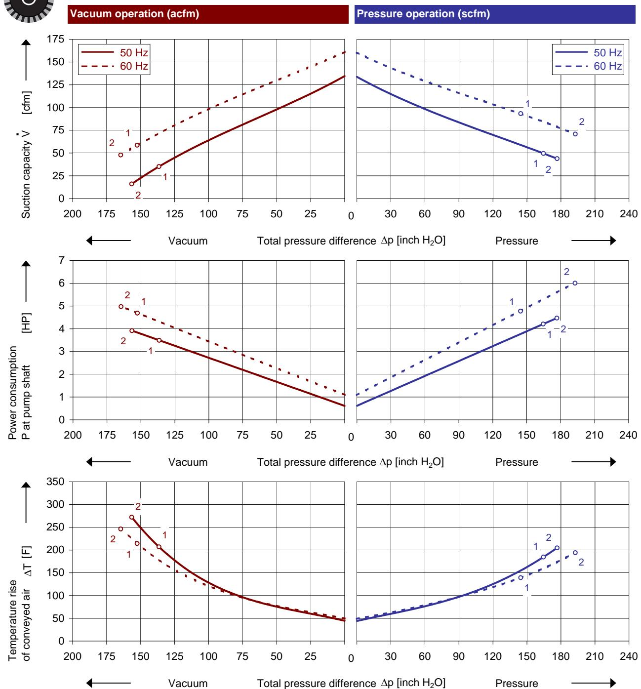
The performance curves are based on air at a temperature of 59 F and an atmospheric pressure of 29.91 inch Hg with a tolerance of  $\pm 10\%$ . The total pressure differences are valid for inlet and ambient temperature up to 77 F. Suction capacity relates to inlet conditions. Pressure capacity relates to atmospheric conditions. For other conditions please get in touch with us.
