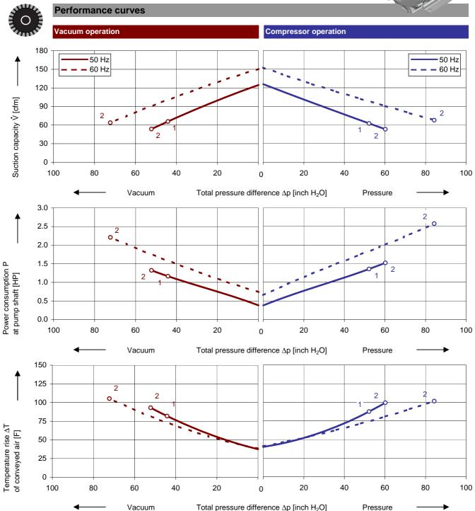
The performance curves are based on air at a temperature of 59 F and an atmospheric pressure of 401.53 inch H2O with a tolerance of  $\pm$  10 %. The total pressure differences are valid for suction and ambient temperature up to 77 F. For other conditions please get in touch with us.
