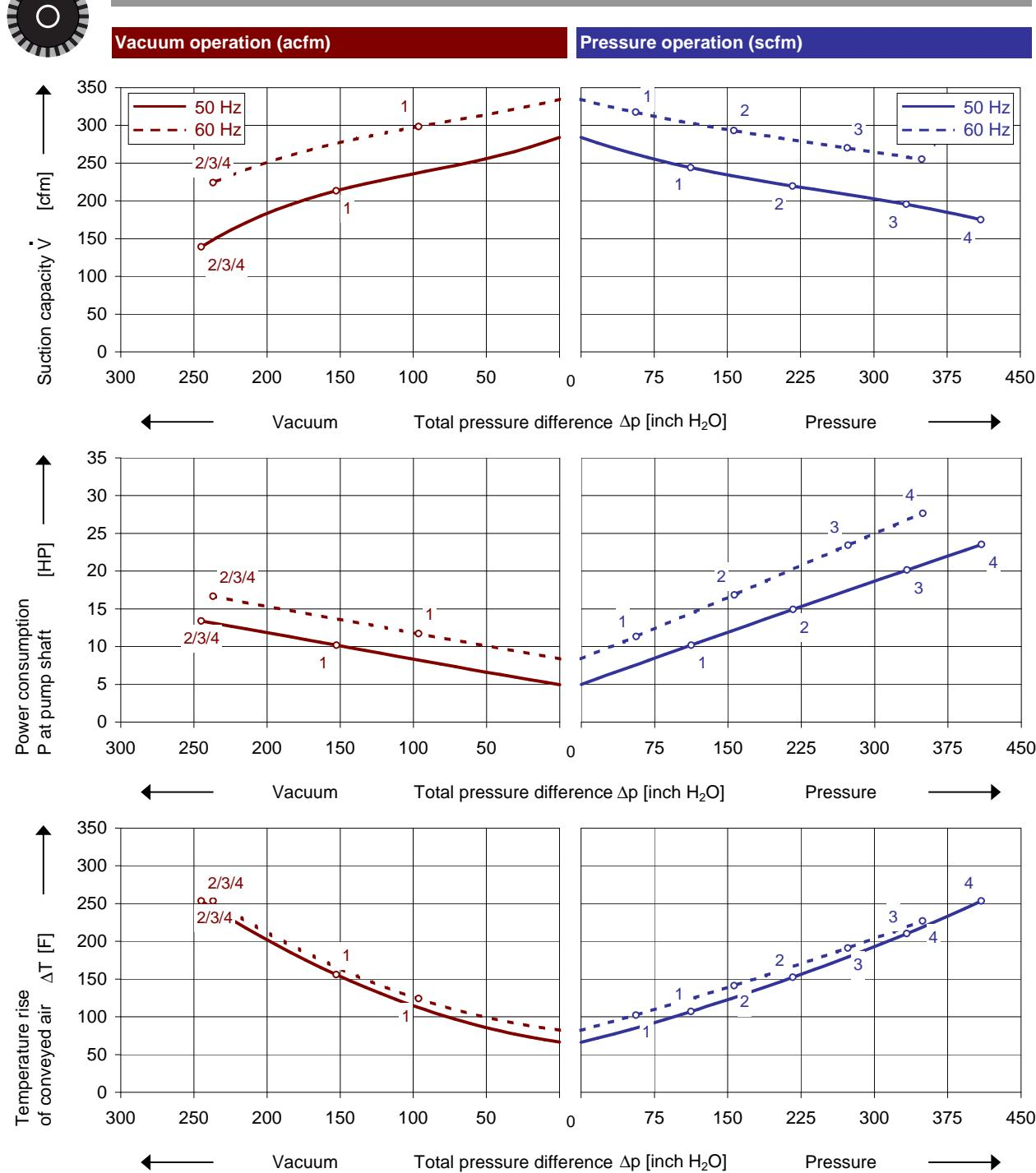
The performance curves are based on air at a temperature of 59 F and an atmospheric pressure of 29.92 inch Hg with a tolerance of  $\pm 10\%$ . The total Suction capacity relates to inlet conditions. Pressure capacity relates to atmospheric conditions. For other conditions please contact Elmo Rietschle.
