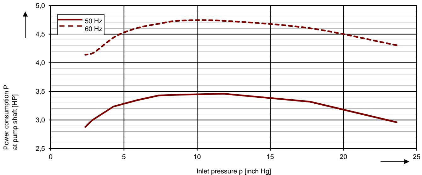
The characteristic curves are based on the evacuation of dry air and an intake temperature of 36 °F. At a suction pressure of 2523 inch. H<sub>2</sub>O abs. (water as operating liquid) the characteristic curves will be achieved. The tolerance is ± 10 %.
