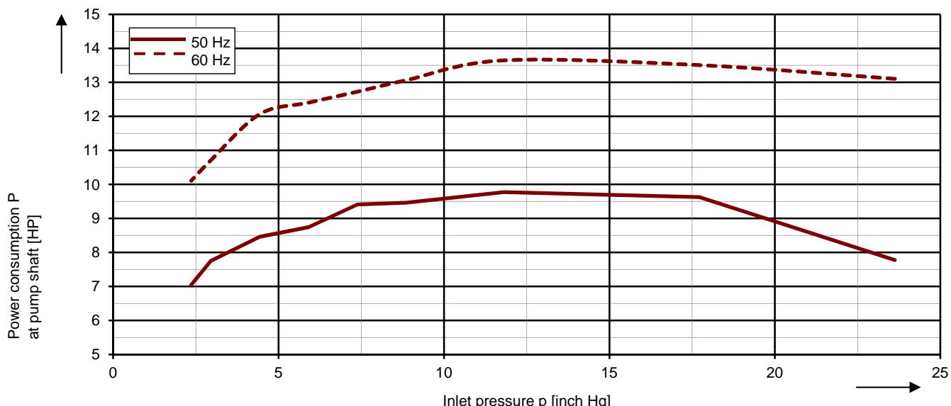
The characteristic curves are based on the evacuation of dry air and an intake temperature of 36 °F. At a suction pressure of 2523 inch. H<sub>2</sub>O abs. (water as operating liquid) the characteristic curves will be achieved. The tolerance is ± 10 %.
