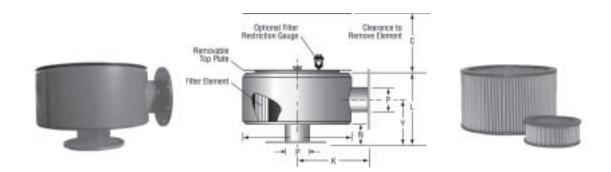
Universal Silencer's new ILFV Series of in-line air filters are designed especially for vacuum applications as an economical alternative to our ILF Series. Choose from ten standard pipe sizes ranging from 2" to 14" and flow capacities ranging from 120 to 5,900 CFM. Two choices of filter element media—pleated paper or pleated felt—are available to suit your specific application.
