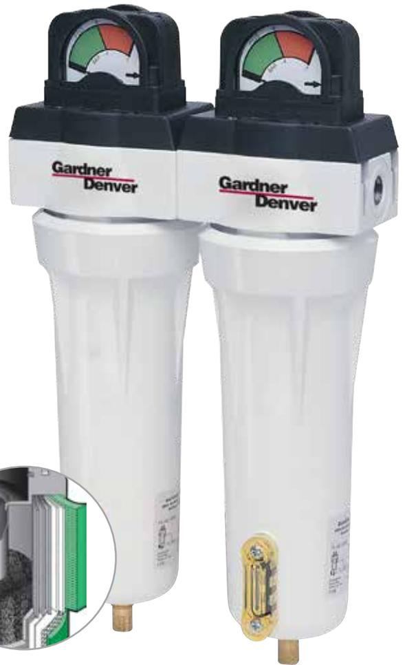
Performance\*\*: No liquid should be present at filter inlet. Provides 0.003 ppm w/w oil (as a vapor) removal and 0.01 micron solid particulate separation.
