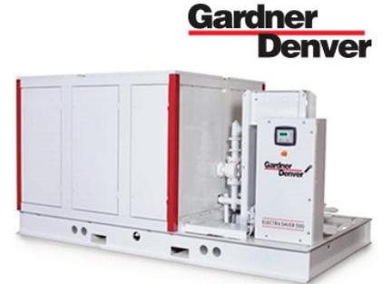
Electra Saver & Electra Saver G2 with infinite positions in an operating range of 40% to 100% capacity, compressor efficiency is maximized because the Turn Valve™ airend compresses only the volume of air required without affecting the built-in compression ratio at partial load conditions.
