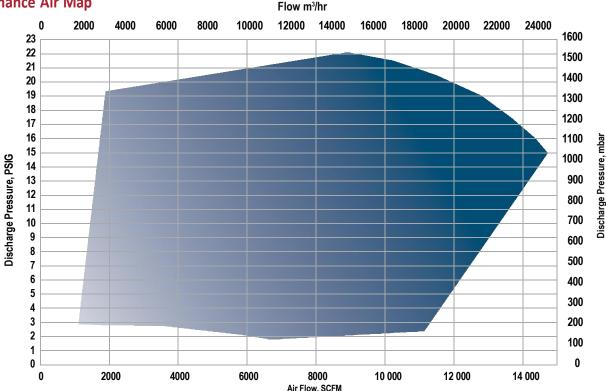
STANDARD CONDITIONS: 14.7 PSIA [1 Bar], 68°F [20°C], 36% RH, Speed: 3550 RPM
